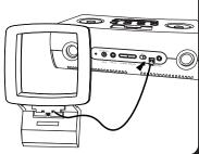
Snap AM antenna into stand, then plug antenna cable into socket on back of ZN9. Move antenna 12" away.
